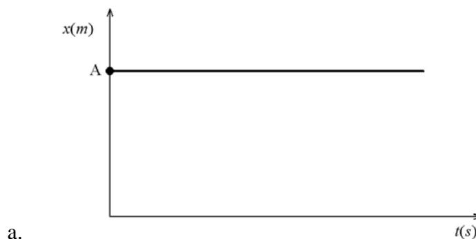
Figure 3.1: The position-time graph of no motion case.
