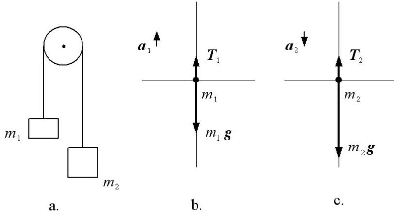
Figure 4.5: a) The Atwood's machine b) the free-body diagram of  $m_1$  and c)  $m_2$ .
