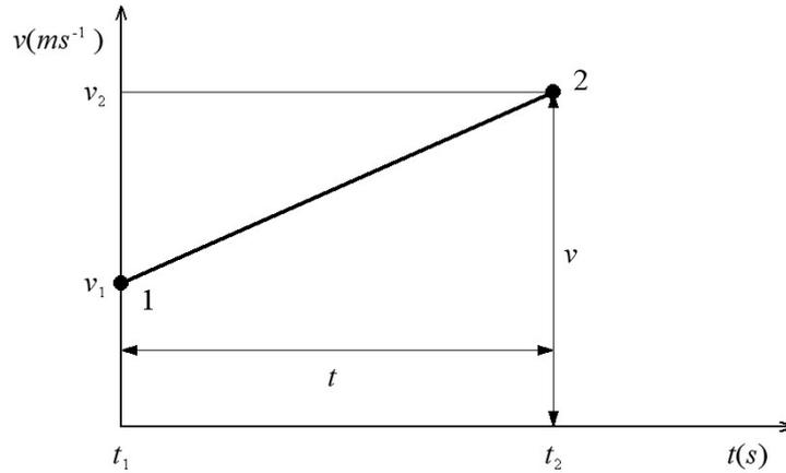
Figure 3.6.b: The velocity-time graph for motion of the particle from the point 1 to the point 2 taking into account the initial conditions.
