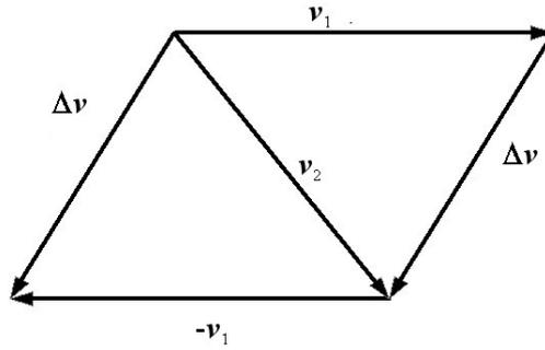
Figure 3.10: The vector analysis of the velocities in circular motion.
