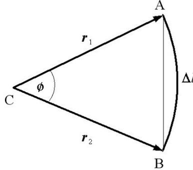
Figure 3.12: The path  $\Delta l$  gone by the particle from the point A to the point B.
