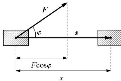
Figure 4.7: The projection of the force  $F$  acting on the body into the direction of the displacement  $s$ .
