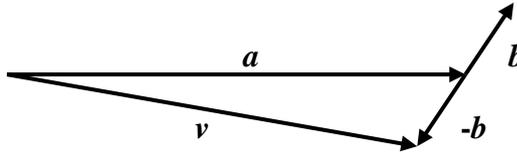
Figure 2.5: The subtraction of two vectors.
