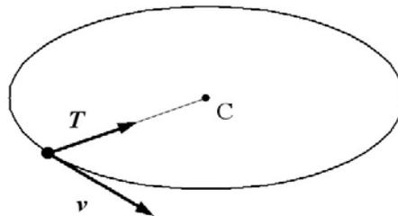
Figure 4.10: The body is attached to a cord and revolving in the horizontal circle.
