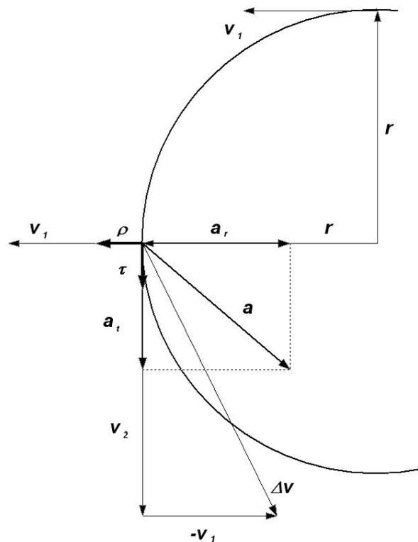
Figure 3.13: The vectors of the velocity and the acceleration in nonuniform circular motion.
