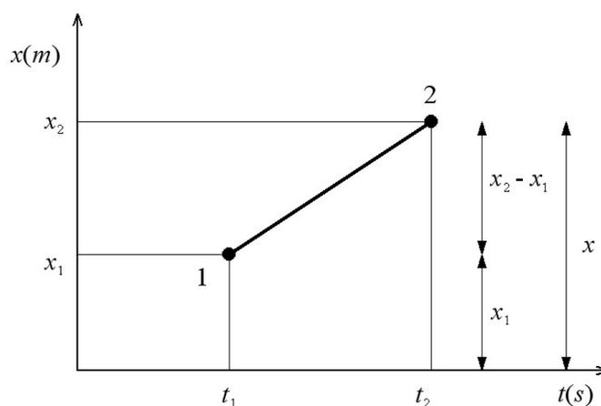
Figure 3.2: The position-time graph of motion at constant speed.
