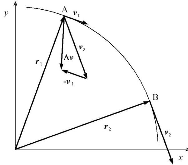
Figure 3.8: The sketch of the velocity vectors in circular motion.
