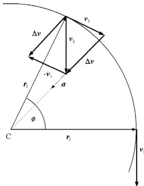
Figure 3.9: Vector analysis of the circular motion of the particle.
