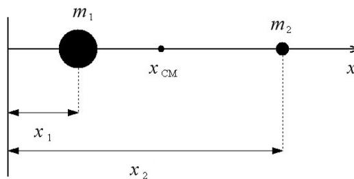
Figure 4.6: The center of mass of the system consisting of two particles.
