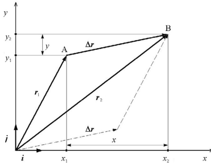
Figure 3.7: The displacement vector  $\Delta\mathbf{r}$  of the particle moving from the point A to the point B.
