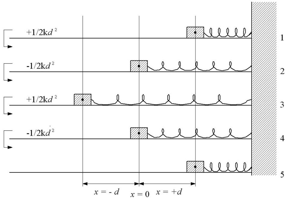
Figure 4.14: Movement of the block of mass attached to the spring.
