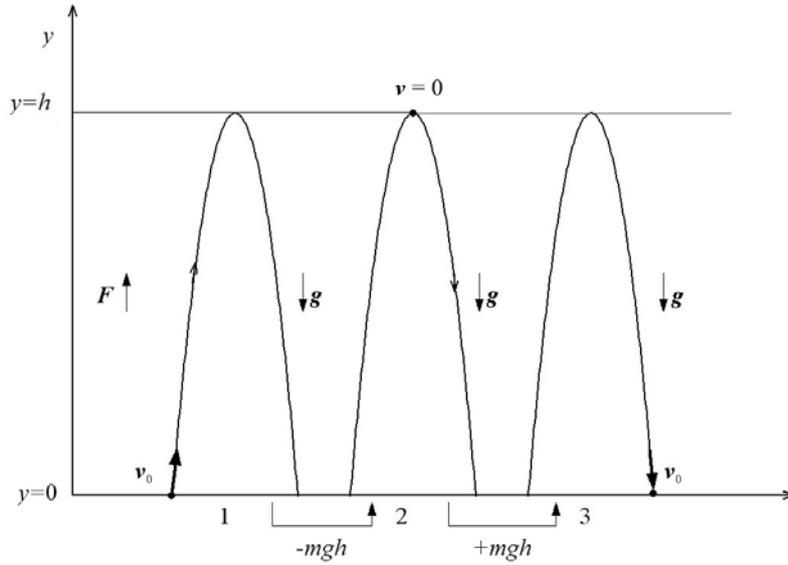
Figure 4.15: The ball is thrown upward (1), stopping in the air (2) and falling down (3).
