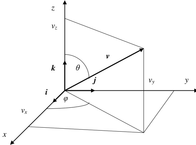
Figure 2.1: The resolving of the vector into its components.
