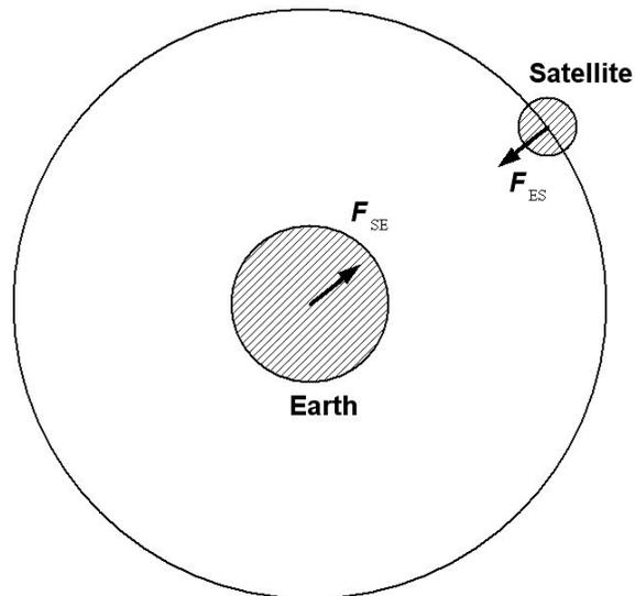
Figure 4.2: The forces of interaction between the Earth and the satellite.
