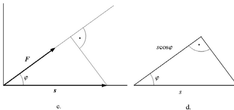
Figure 4.12: The projection of the displacement  $s$  of the body in the direction of the force  $F$ .
