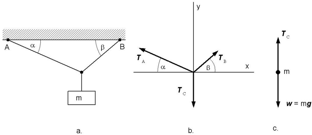
Figure 4.3: a) A block of mass hangs from three strings A, B and C, b) free-body diagram of the knot that joins the strings, c) the free-body diagram of the block.
