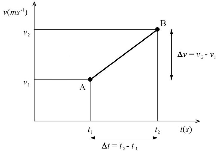
Figure 3.5: The velocity-time graph of motion of the particle moving from the point A to the point B.
