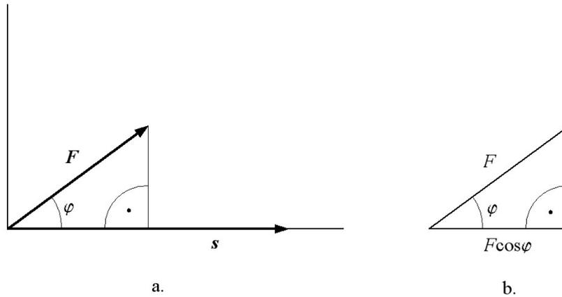
Figure 4.11: The projection of the force  $F$  acting on the body in the direction of the displacement  $s$ .
