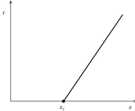
Figure 3.15: The position-time graph of the linear motion.
