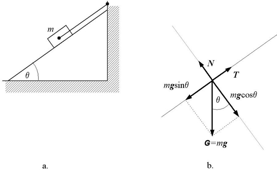
Figure 4.4: a) The block of mass on the inclined plane and b) the free-body diagram of the block of mass.
