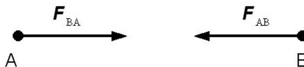
Figure 4.1: The forces of interaction between two particles.
