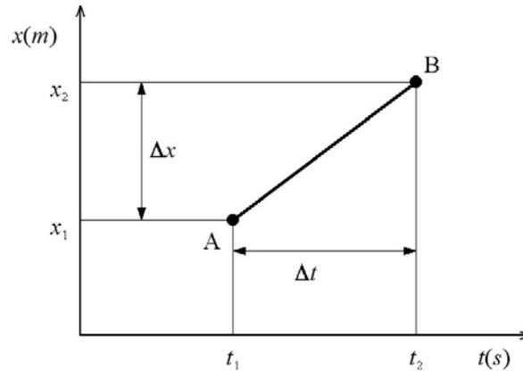
Figure 3.4: The position-time graph of the particle moving from the point A to the point B .
