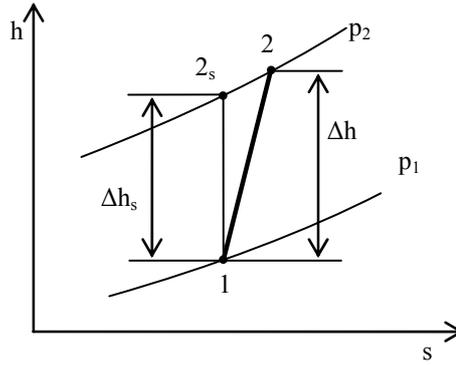
Fig. 1 Static thermodynamic change behaviour in gas compressor.
