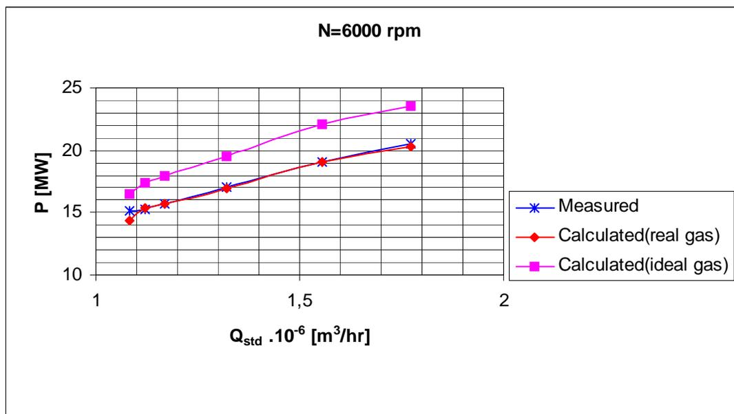
Fig. 4 Absorbed compressor power (N=6000 rpm,  $t_1 \sim 13,8^\circ\text{C}$ ,  $p_1 \sim 4,9\text{MPa}$ ,  $p_2/p_1 = 1,436-1,4865$ ).
