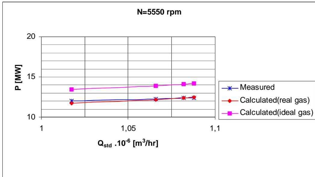
Fig. 5 Absorbed compressor power ( $N=5550$  rpm,  $t_1 \sim 13,8^\circ C$ ,  $p_1 \sim 4,97 MPa$ ,  $p_2/p_1 = 1,406-1,40926$ ).
