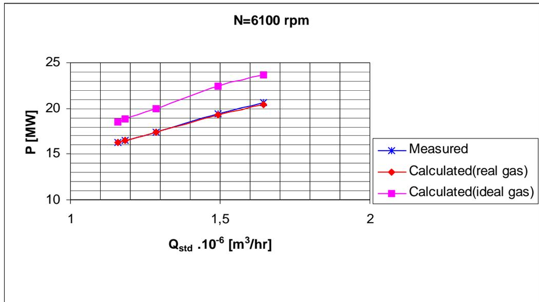
Fig. 3 Absorbed compressor power (N=6100 rpm,  $t_1 \sim 13,8^\circ\text{C}$ ,  $p_1 \sim 4,9\text{MPa}$ ,  $p_2/p_1 = 1,48-1,50263$ ).
