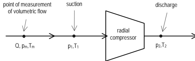
Fig. 2 Points of measurement.
