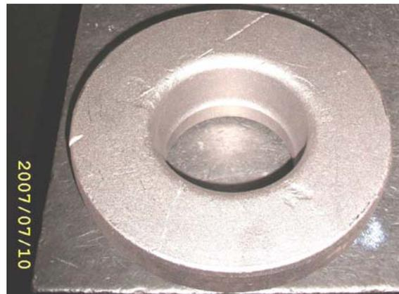
Fig.18 Flange stub from trial production.
