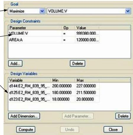
Fig.8 Modified blank dimensions /  $V=999380 \text{ mm}^3$   $A=119999 \text{ mm}^2$  /.
