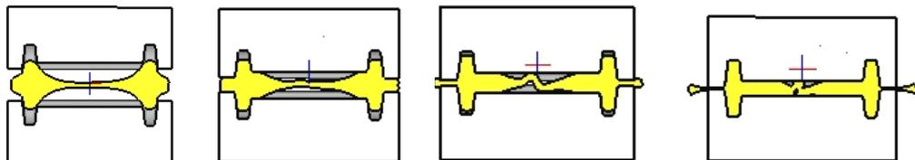
Fig.1 Fold and lap in die forging.
