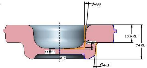
Fig.14 Changed angles and / or heights of the basic body.
