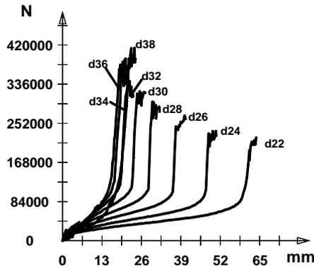
Fig.10 Diagram of force vs. stroke with blanks of various diameters and constant volume.
