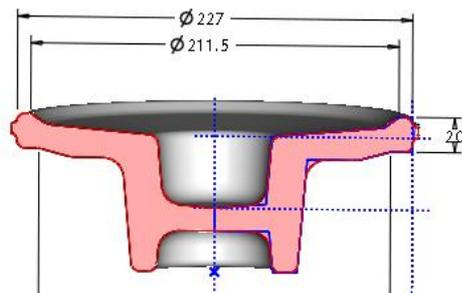
Fig.7 Selected blank dimensions /  $V=999378$
