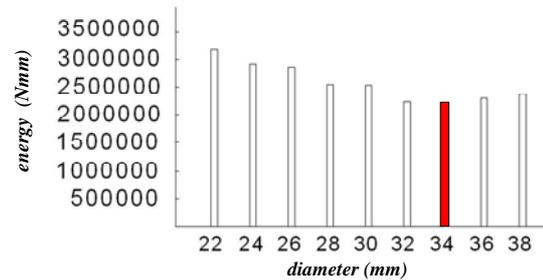
Fig.11 Work required in forming blanks of various diameters and constant volume.
