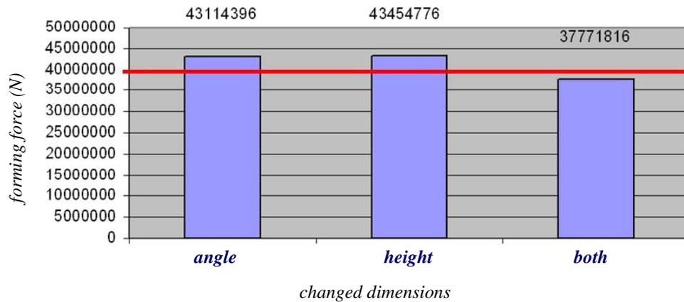
Fig.16 Force required in forming various blanks pre-upset to 65 mm.
