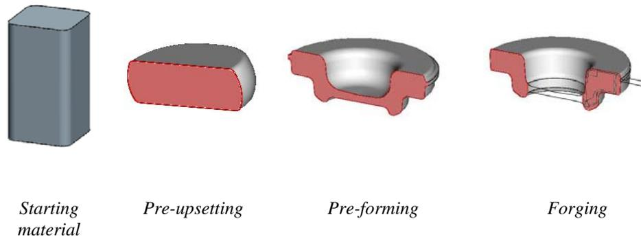
Fig.12 Multiple-cavity forging of flange stub.
