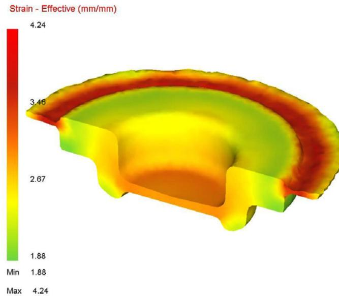
Fig.17 Strain distribution in finish-forming the flange stub.
