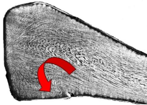
Fig. 5 Detection of grain fold with etching the cross-section on one side of the ring gear support.
