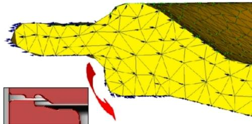
Fig.6 Velocity vectors of material flow.
