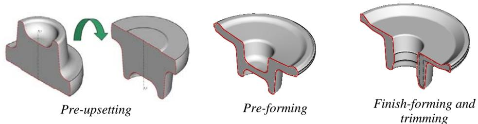
Fig.3 Intermediate parts of ring gear support.
