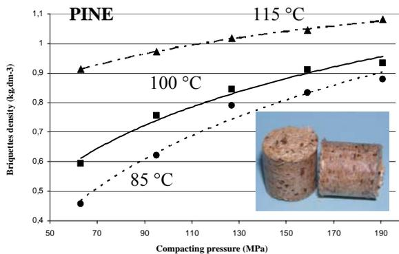
Fig. 8 Dependence of briquettes density from pine sawdust from compacting pressure by various pressing temperatures ( $w_r=10\%$ ;  $L=2\text{mm}$ ) [5].
