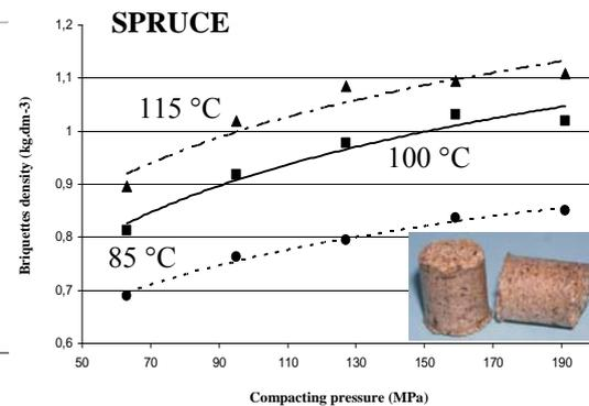
Fig. 9 Dependence of briquettes density from spruce sawdust from compacting pressure by various pressing temperatures ( $w_r=10\%$ ;  $L=2\text{mm}$ ) [5].
