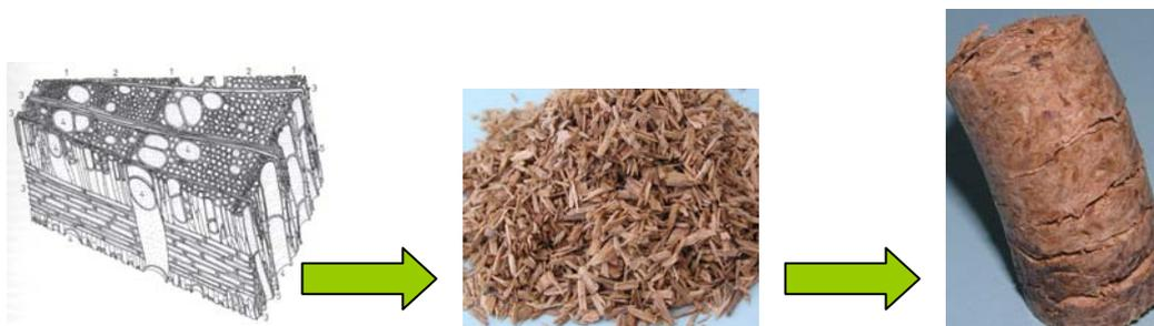
Fig. 5 Three-dimensional cross-section of hardwood – beech (left), beech sawdust (in the middle) prepared for pressing and pressed briquette from beech sawdust (right) [3]; [6].
