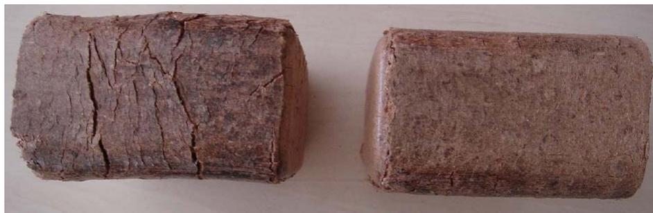
Fig. 3 Examples of ashlar shaped wood briquettes pressed from materials with different moisture content (left approx. 18 %, right approx. 10%).
