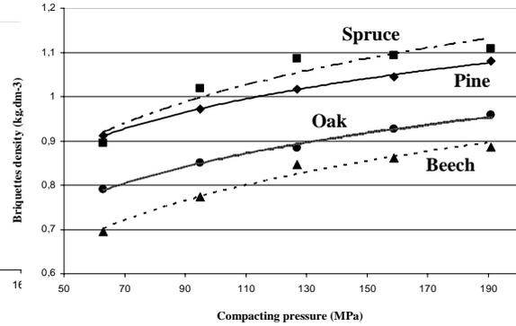
Fig. 7 Comparison of dependencies of briquettes density from various materials from compacting pressure by pressing temperature 115 °C ( $w_r=10\%$ ;  $L=2\text{mm}$ ) [5]; [6].
