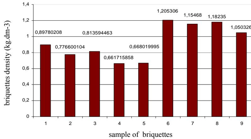
Fig. 1 Comparison of some briquettes density from various types of materials: 1-mixed municipal waste (wood 38%, paper 45%, PET bottles 11%, textile 6%); 2-RDF with addition of 20% of disintegrated carton waste; 3-RDF with addition of 4% of cement; 4-RDF with addition of 20% of wood sawdust; 5-Clear RDF; 6-Softwood; 7-Cacao cracks; 8-Hardwood; 9-Corn straw [1], [2].
