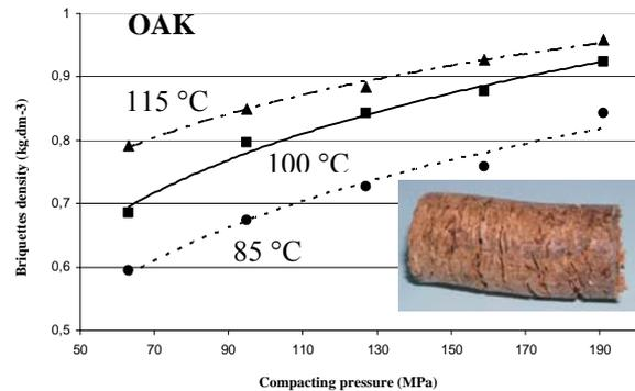
Fig. 11 Dependence of briquettes density from oak sawdust from compacting pressure by various pressing temperatures ( $w_r=10\%$ ;  $L=2\text{mm}$ ) [5].
