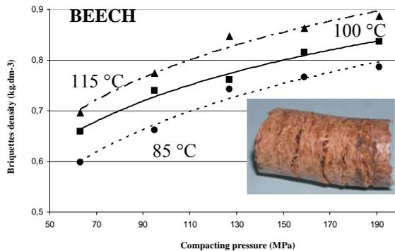
Fig. 10 Dependence of briquettes density from beech sawdust from compacting pressure by various pressing temperatures ( $w_r=10\%$ ;  $L=2\text{mm}$ ) [5].
