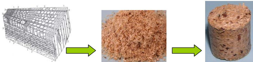
Fig. 4 Three-dimensional cross-section of softwood – pine (left), pine sawdust (in the middle) prepared for pressing and pressed briquette from pine sawdust (right) [3]; [6].
