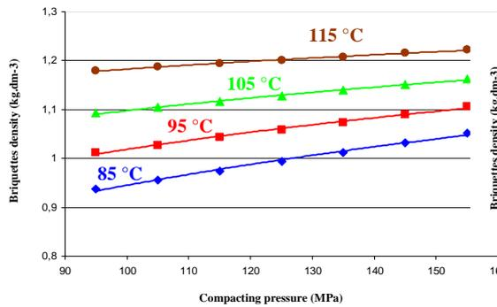
Fig. 6 Dependence of briquettes density on compacting pressure by various pressing temperatures for pine sawdust ( $w_r=10\%$ ;  $L=2\text{mm}$ ) [1].
