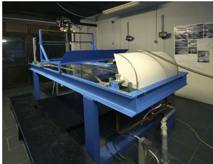
Fig. 1 Low-level hydrodynamic tank.
