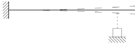
Fig. 3: Measuring of amplitude of vibration by optical sensor
