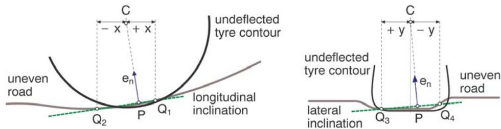
Fig. 3 Track normal and geometric contact point on uneven roads.
