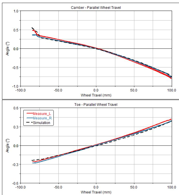
Fig. 6 Camber and toe angles during parallel wheel travel from simulations and measurements.
