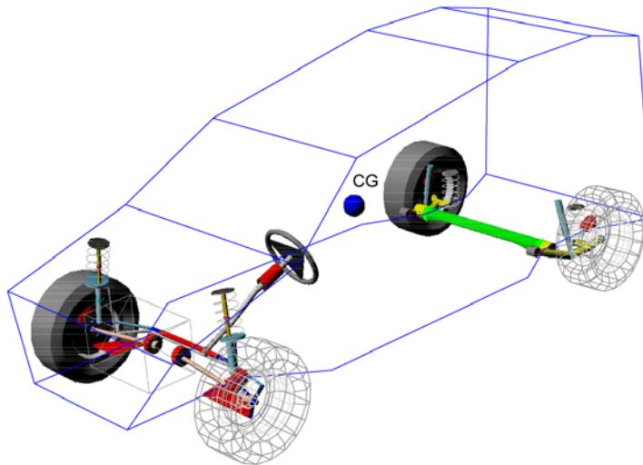
Fig. 1 MBS full model of the vehicle.
