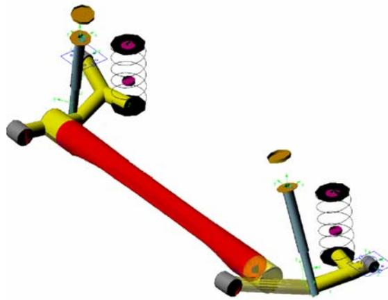
Fig.2 Rear suspension model.
