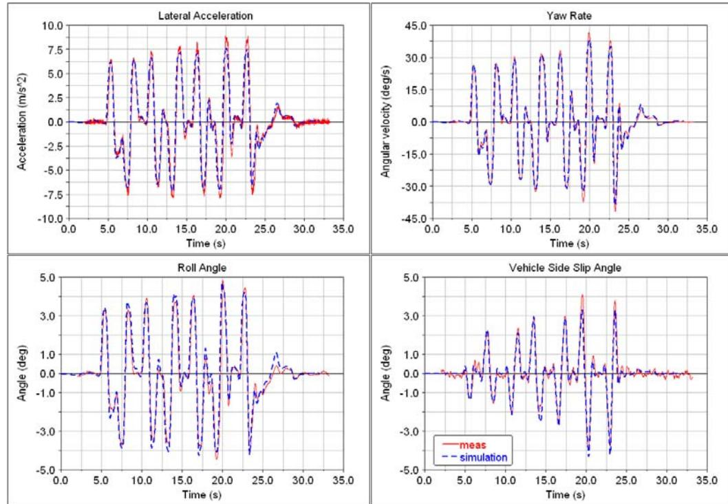
Fig. 7 Comparison simulation-measurement: Multiple lane change.
