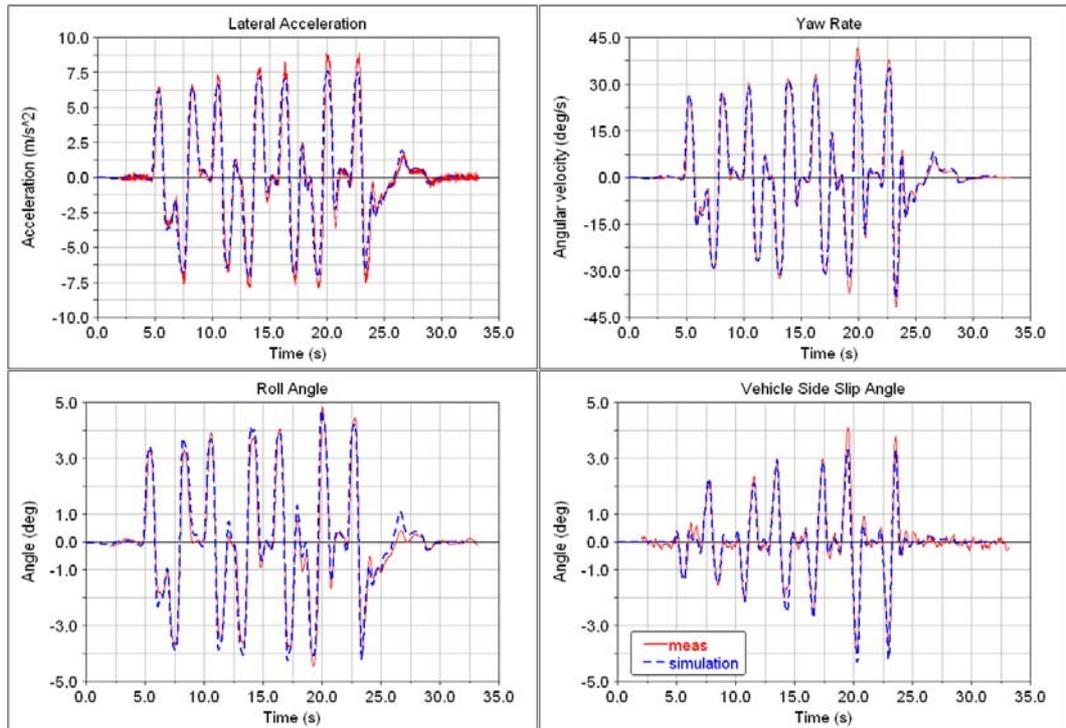
Fig. 7 Comparison simulation-measurement: Multiple lane change.
