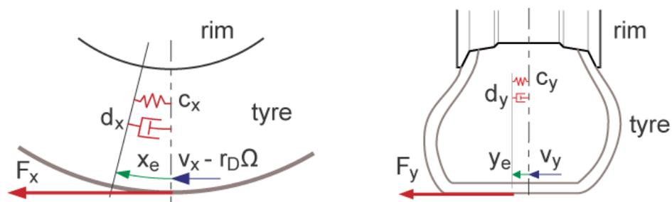
Fig. 4 Tyre deflection in longitudinal and lateral direction.
