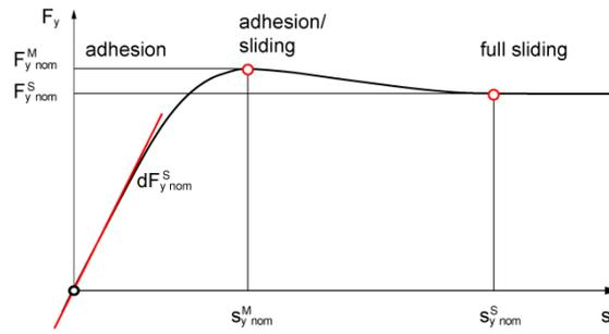
Fig. 5 Lateral force function with five parameters for  $F_{z,nom}$ .
