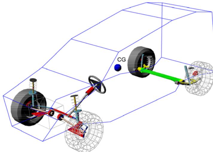
Fig. 1 MBS full model of the vehicle.
